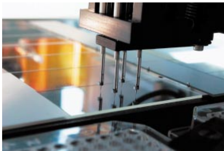
Figure 2 Genetic Microsystems' (GMS) 417 "pin and ring" spotting robot.
